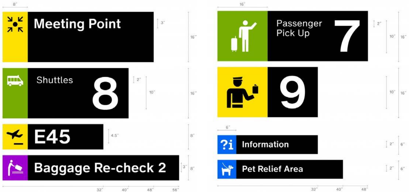
Various suspended or wall-mounted signs in both 8- and 6-inch scales
