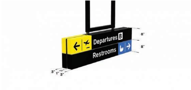
Sign box showing typical dimensions.
